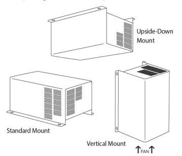
The location should be selected to prevent excessive heat, water, moisture, dust and dirt entering the unit installed. As a rule, allow two cubic feet of clear airspace and or any additional venting as necessary to prevent the unit from overheating. The front of the enclosure should not be obstructed to allow free air flow for the cooling fan (above).
