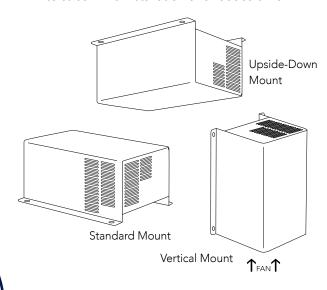
This versatile deck mount converter can be installed in any position, making RV design more flexible for manufacturers.
