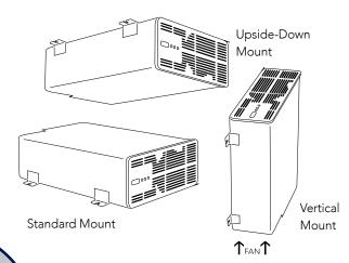
WFCO recommends horizontal mounting of the WF-68100AD series. You can mount it in any position that provides unobstructed ventilation for the fan and vent holes.
